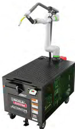
Cooper CRX-10iA/L Air-Cooled Wire-Break Welding Cobot Cart
