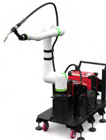
Cooper CRX-25iA Air-Cooled Wire-Break Welding Cobot Cart
