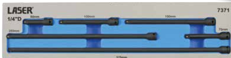
7371 Impact Extension Bar Set 1/4"D 6pc Lengths: 50, 75, 100, 150, 250 and 375mm.
