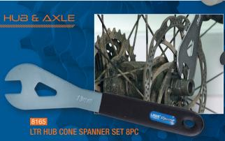
Typically 5mm thinner than a regular spanner, cone nut spanners slide between the hub and the axle locking nut, onto the cone nut to allow for the hub bearings to be correctly adjusted. This set of cone nut spanners is ideal for use by both the home or shop mechanic.
